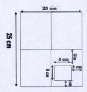
(b) Determine the centroid of the lamina shown in fig:
