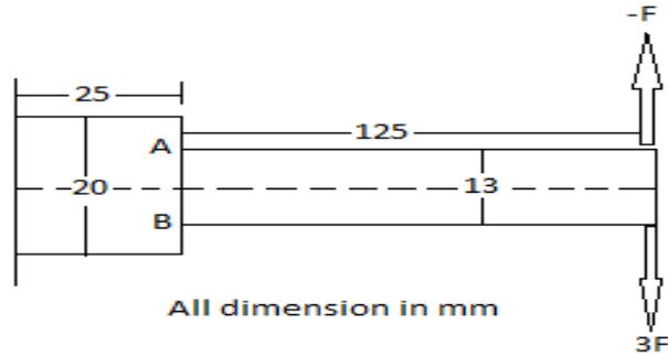
Q3. A forged steel bar 50 mm in diameter, is subjected to reversed bending stress of 250 N/mm<sup>2</sup>. The bar is made of steel 40C8 ( $S_{ut} = 600 \text{ N/mm}^2$ ). Calculate the life of the bar for a reliability of 90%. Assume the Following values- [ $k_a=0.44$ ,  $k_b=0.85$  &  $k_c=0.897$ ].
