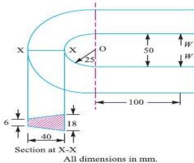
Q6 A C-clamp is subjected to a maximum load of  $W$ , as shown in Fig. If the maximum tensile stress in the clamp is limited to  $140 \text{ Mpa}$ , find the value of load  $W$ .
