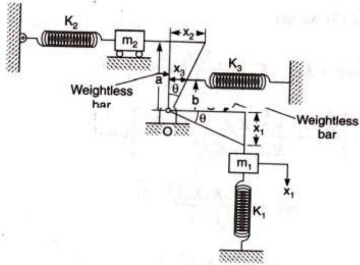
Q 4 Determine the natural frequency of the system by energy method (Shown in displaced position)
