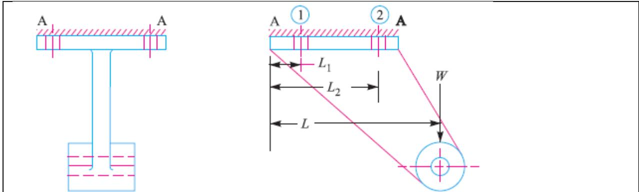
9. Determine the size of the bolts and the thickness of the arm for the bracket as shown in Fig, if it carries a load of 40 kN at an angle of  $60^\circ$  to the vertical. The material of the bracket and the bolts is same for which the safe stresses can be assumed as 70, 50 and 105 MPa in tension, shear and compression respectively.
