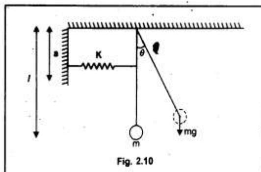
Q3 Determine the natural frequency of the system by energy method (Shown in displaced position)
