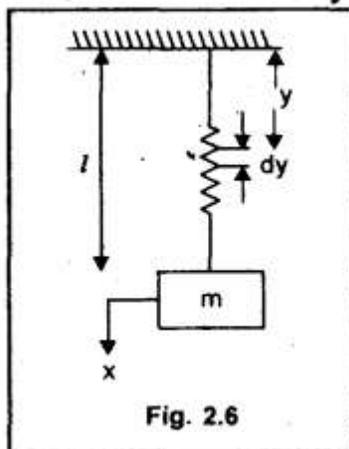
Q. 2 Determine the natural frequency of spring controlled simple pendulum as shown in Fig.
